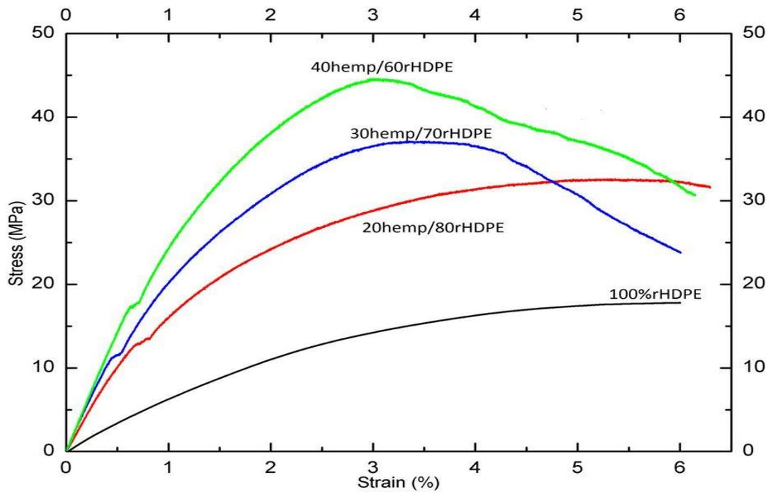
**Figure 3:** Flexural stress of hemp/rHDPE composite at various fiber fraction along with pure rHDPE (Lu and Korman, 2013).
